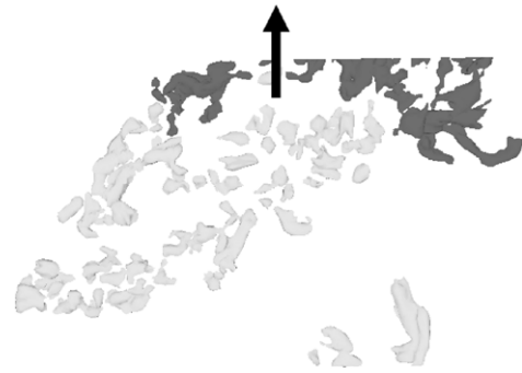
Fig. 4. Distribution of extracted components. The finished components are shown in light gray and growing ones in dark gray. The black arrow indicates the direction used for extraction.
